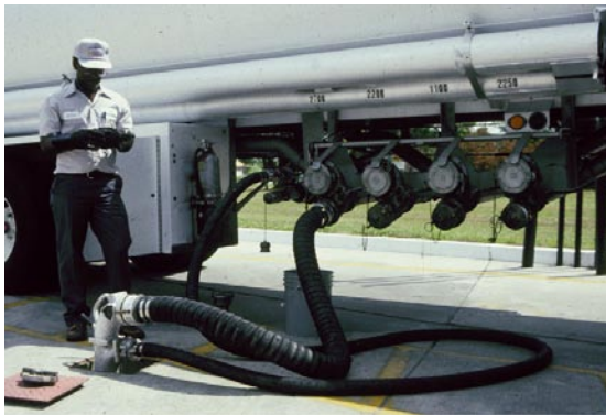
Figure 2. Coaxial Stage I vapor recovery is easy to retrofit to existing tanks because it usually does not require breaking concrete. However, because the diameter of the drop tube is reduced, the delivery flow rate is slower and the time required to make a delivery is increased.
